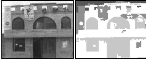
Fig. 5. A 94 \times 115 intensity image (left) and its segmentation (right). Parameter setting: \sigma = 0.15 . Minimal region size of interest is 11
