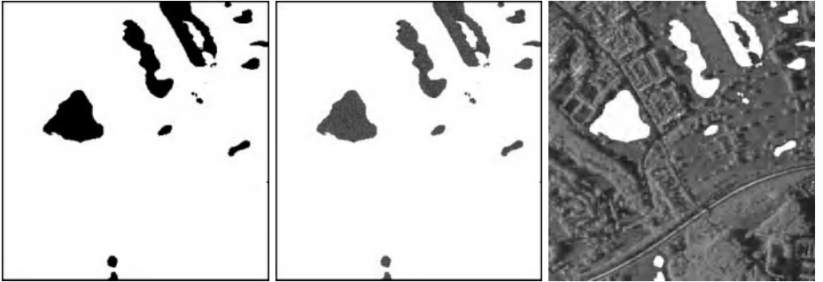
Fig. 14. Segmentation of the SAR image of terrain using the threshold related to the distance distribution for the training patch, the regions similar to the patch, and the background region
